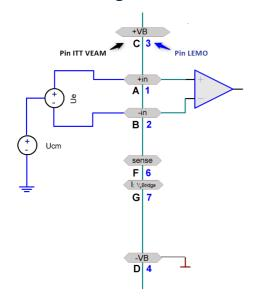
The common mode voltage ( $U_{cm}$ ) has to be less than  $\pm 10$  V. It is reduced by  $\frac{1}{2}$  input voltage.
