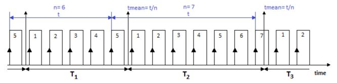
The frequency is determined as the number of events counted divided by the time between the first and the last "complete" event in the interval. An event is complete when a positive edge is succeeded by a subsequent positive edge.
