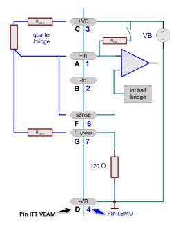
A quarter bridge can consist of a single strain gauge resistor, whose nominal value can be 120  $\Omega$  or 350  $\Omega$ . C-70xx internally completes an additional 120  $\Omega$  that can be switched to a 350  $\Omega$  quarter bridge.
