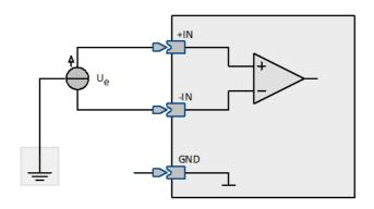
The voltage source itself already is referenced to the device's ground. The voltage source is at the same potential as the device ground.
