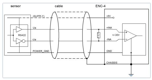
sensor with RS422 differential output
