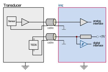
A Class II Mixed Mode Interface receives/ sends TEDS data and analog signals on different lines. The sensor is not influenced.
