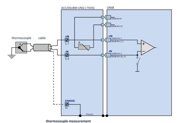
It is not a problem if the ground potential at the thermocouple differs from that of the device units by a few volts. However, the maximum allowed common mode voltage may not be exceeded.
