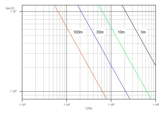
Maximum signal amplitudes as a function of the signal frequency and the cable length, with a 4 mA feed and a capacitance of 100 pF/m.
