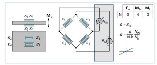
The sensitivity of the bending moment is increased. At the same time, longitudinal force, torque and temperature are compensated for.
