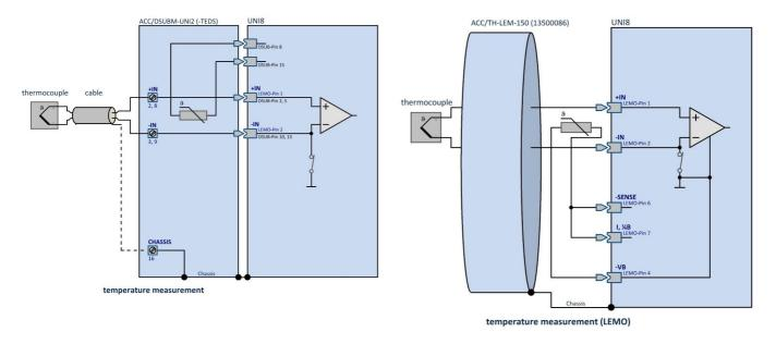
In the operating software, activate "*Isolated thermo couple*" at the amplifier tab. In this measurement mode, the unit itself provides the ground reference by having Terminals -IN and -VB connected internally. This connection is only made in the Thermocouple mode and not with voltage measurements.
