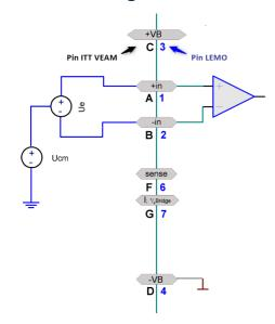
The common mode voltage ( $V_{cm}$ ) has to be less than  $\pm 10$  V. It is reduced by ½ input voltage.
