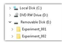
To perform **formatting of a storage medium via the Windows-Explorer** 28, navigate to the desired storage medium. Run the formatting by means of the context menu, for example.
