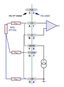
The PT100 is supplied with constant current via two lines (-SENSE and -VB). Another line (I, 1/4B) measures the voltage across the supply line and uses it to compensate for parasitic voltage drops. It is assumed that the resistances of the supply lines have the same size and the same temperature drift.
