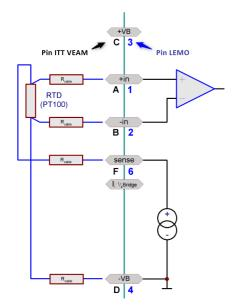
The PT100 is supplied with constant current via two lines (-SENSE and -VB). The other two serve as Sense-leads. By using the lines (+IN und -IN), the voltage at the resistor itself can be determined precisely. The voltage drop along the conducting cable thus does not cause any measurement error. The 4-wire configuration is the most precise way to measure with a PT100.
