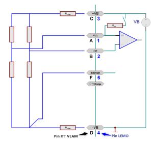
Please note that the maximum allowed voltage drop along a cable may not exceed approx. 0.5 V. This determines the maximum possible cable length.
