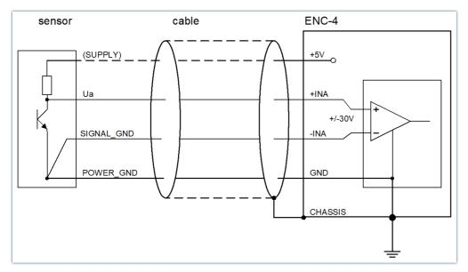
sensor with open-collector output
