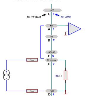
In this circuit, the current to be measured flows through the 120  $\Omega$  shunt in the amplifier. Note that here, the terminal -VB is simultaneously the device's ground. Thus, the measurement carried out is single-ended or ground referenced. The potential of the current source itself may be brought into line with that of the units ground. In that case, be sure that the device unit itself is grounded.
