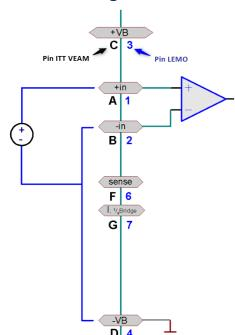
The voltage source itself is not referenced to the amplifier ground but is instead isolated from it. In this case, a ground reference must be established. One way to do this is to ground the voltage source itself. Then it is possible to proceed as for Voltage source with ground reference 128. Here, too, the measurement is differential. It is also possible to make a connection between the negative signal input and the device ground, in other words to connect -IN and -VB.
