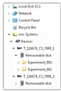
While installing the operating software, if the option "Extension for Windows-Explorer" is activated, you are able to copy, display or delete the files of measured data saved within the device (e.g. on the removable storage medium). The method of doing this is the familiar one under Windows.
