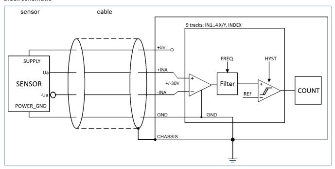
Dual-track encoders (quadrature encoders) emit two signals offset by 90° of phase, the tracks A and B. By evaluating the phase information between the A and B-track, the direction of turning can be determined. If the corresponding encoder type is selected, this functionality is supported. The actual time or frequency information, however, is derived exclusively from the A-track!
