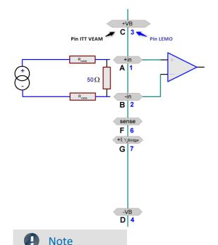
For current measurement the DSUB plug ACC/DSUBM-I2 is mandatory. The ACC/DSUBM-I2 comes with a 50  $\Omega$  shunt and is not included with the standard package. It is also possible to measure a voltage via an externally connected shunt. Appropriate scaling must be set in the user interface. The value 50  $\Omega$  is just a suggestion. The resistor needs an adequate level of precision. Pay attention to the shunt's power consumption.
