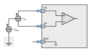
In the input ranges <20 V, the common mode voltage Ucm must lie within the range ±10 V. It is reduced by one-half of the input voltage.
