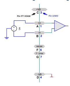
The voltage source itself already has a connection to the device's ground. The potential difference between the voltage source and the device ground must be fixed.
