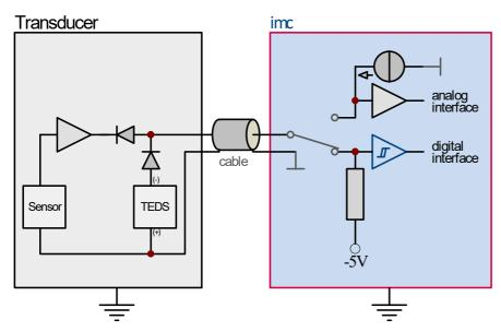
A Class I Mixed Mode Interface receives/ sends TEDS data and analog signals on the same line
