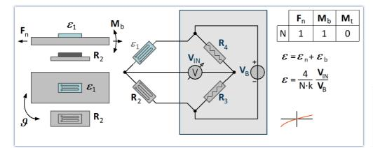
The configuration does compensate the thermal influence (*insensitive to temperature changes*).
