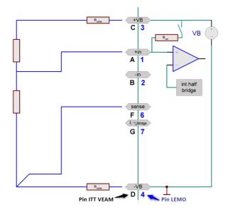
A half bridge may consist of two strain gauges in a circuit or a sensor internally configured as a half bridge, or a potentiometer sensor. The half bridge has 4 terminals to connect. For information on the effect and use of the SENSE lead, see the description of the <u>full bridge</u> 130.
