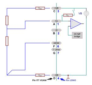
A half bridge may consist of two strain gauges in a circuit or a sensor internally configured as a half bridge, or a potentiometer sensor. The half bridge has four terminals to connect. For information on the effect and use of the Sense lead SENSE, see the description of the full bridge.
