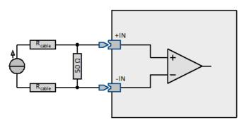
In this configuration, too, the maximum common mode voltage must be located within the range: ±10 V. This can generally only be assured if the current source is also already referenced to ground.
