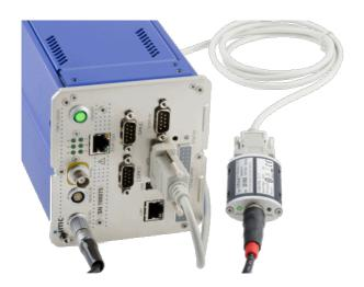
The IRIG-B module comprises a realtime clock (RTC) with a backup battery, which is set to time and date according to the IRIG B-signal received. If the IRIG B year codes received equal "00" (depending on used sub-standard) these are ignored and only RTC time and day values are set, while the year continues to reflect the value resulting from counting since the last update with a valid year number. This means that the year number is incremented at the turn of the new year.
