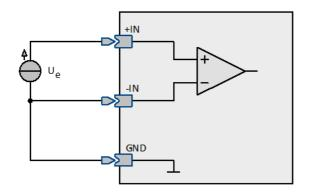
The voltage source itself has no reference to the device's ground, but instead, its potential floats freely compared to the device ground. If a ground reference cannot be established, it's also possible to connect the negative signal input –IN to the ground contact GND.
