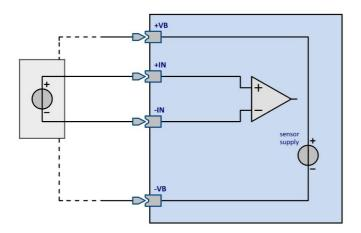
The sensor supply is unipolar and can be led out with DSUB-15 plugs at +VB and -VB (or +SUPPLY and -SUPPLY, see typing label in your plug). Only five selectable settings are available per module. The configurations can be taken from the respective module data sheet. The voltage can be set globally for all channels of a module. All channels of a module form a channel group.
