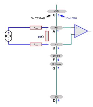
For current measurement could be used the DSUB plug ACC/DSUBM-I2. That plug comes with a 50  $\Omega$  shunt and is not included with the standard package. It is also possible to measure a voltage via an externally connected shunt. Appropriate scaling must be set in the user interface. The value 50  $\Omega$  is just a suggestion. The resistor needs an adequate level of precision. Pay attention to the shunt's power consumption.
