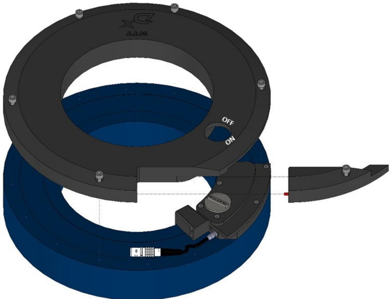
Fig. 24: WTT with battery and loosened partial cover (exploded view)
