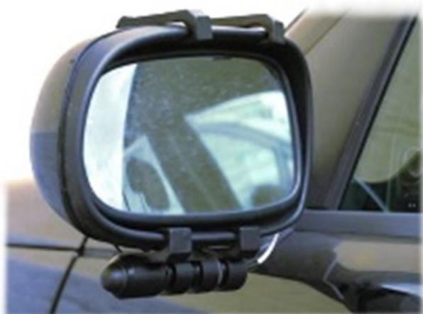
Fig. 4: antennas for the mirror
