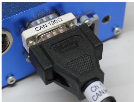
Fig. 13: Plugged CAN terminating resistor
