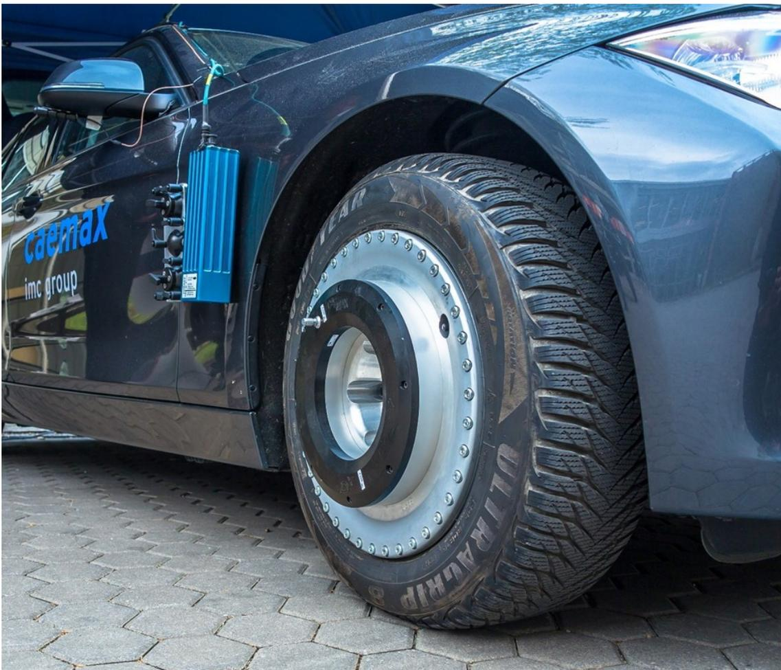
Fig. 10: Installed WTT
