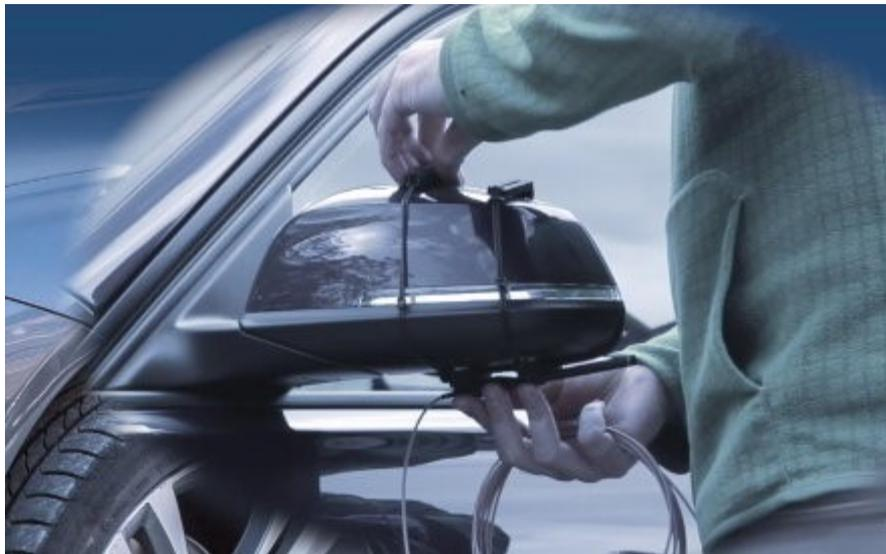
*Fig. 11: Attach the mirror antennas*
