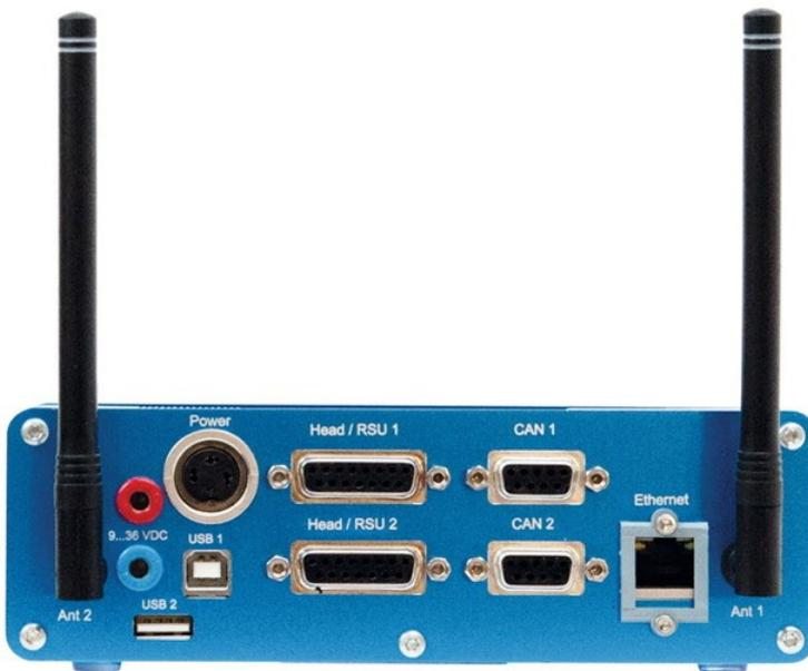
Fig. 3: Dx-RCI (sockets rear side)
