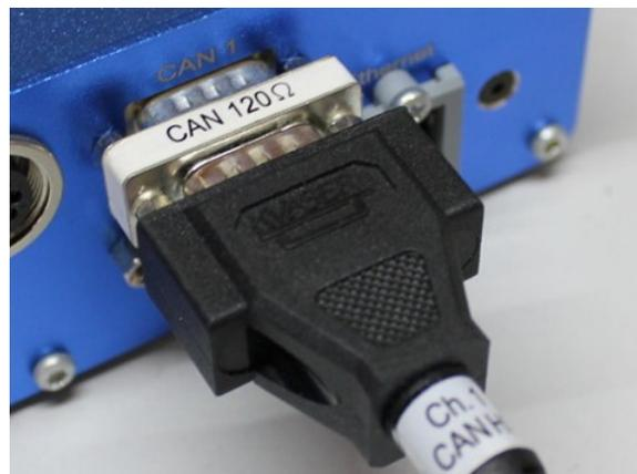
Fig. 18: Plugged CAN terminating resistor
