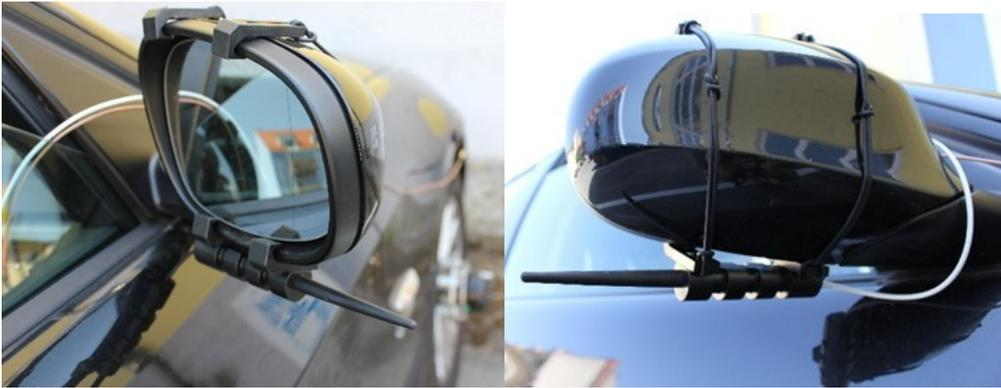
*Fig. 28: Antennas for the exterior mirror of a car (front and rear)*
