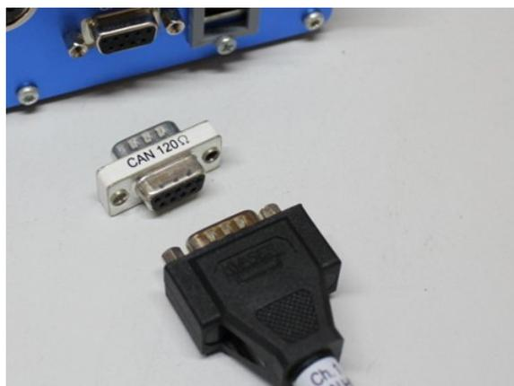
Fig. 12: CAN terminating resistor
