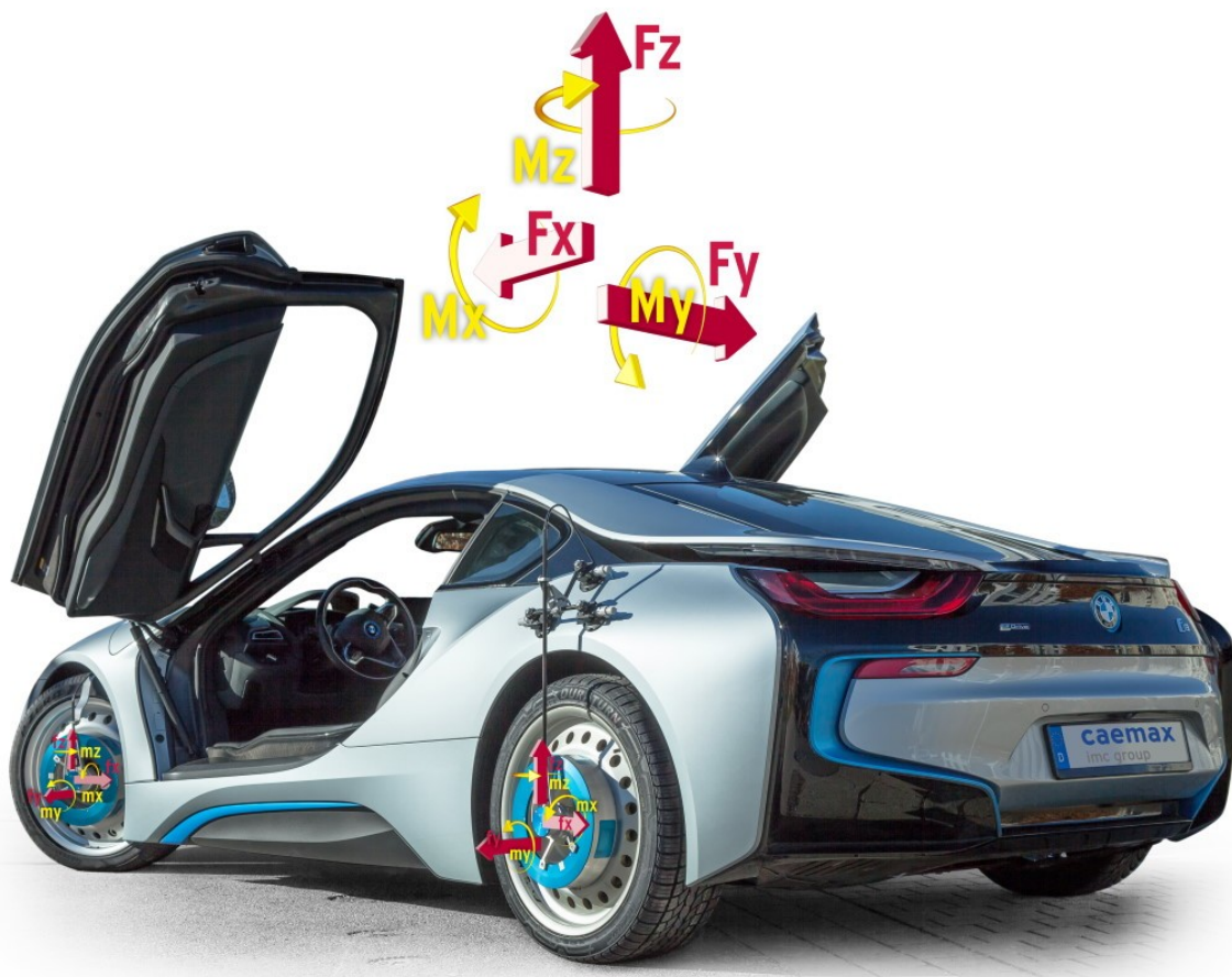
Fig. 22: i8 with WFT-C x mounted on front and rear wheel
