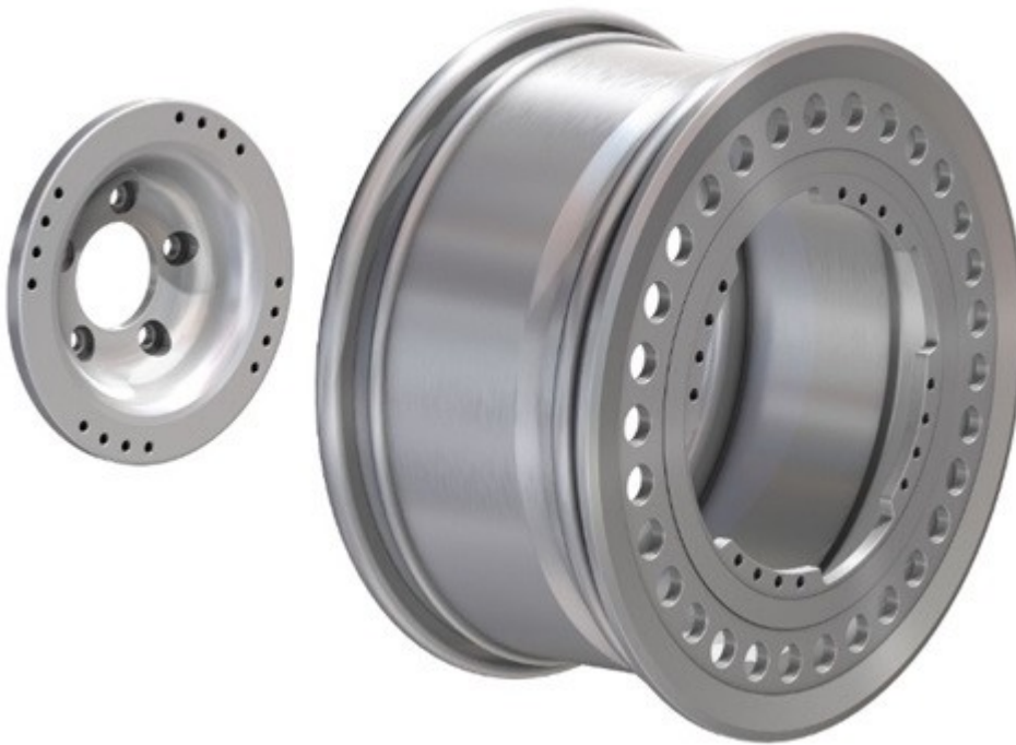
Fig. 9: WFT hub adaptor (left) and modified rim (right)
