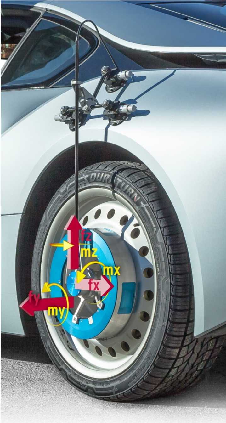
Fig. 20: Stator connection to the WFT, rear wheel (example photo)
