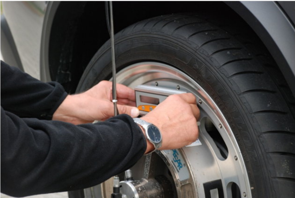
Fig. 28: Measuring with the bubble level
