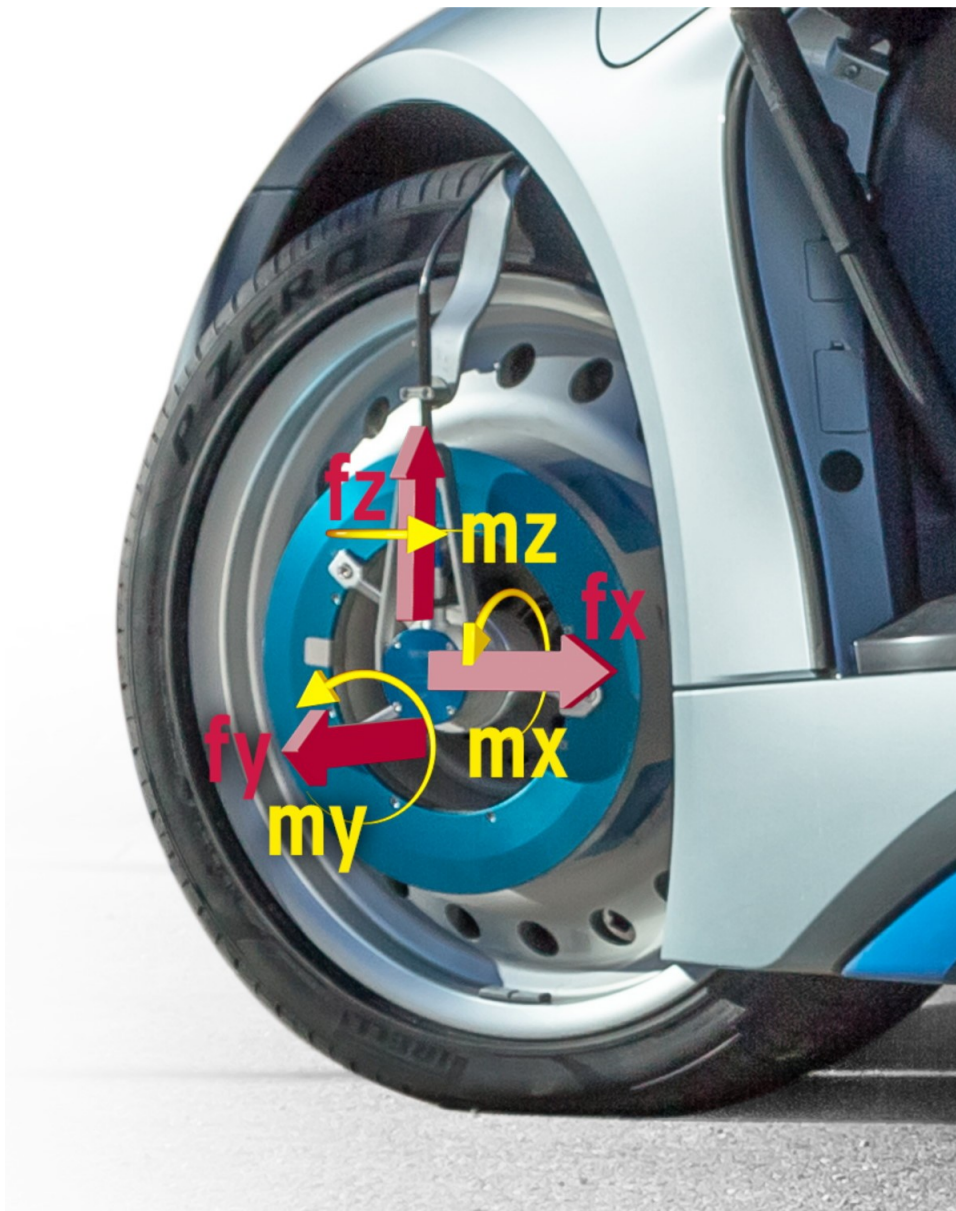
Fig. 21: Stator connection to the WFT, front wheel (example photo)
